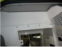
Install ceiling filler panel to passenger side of K9 housing using <sup>1</sup>/<sub>4</sub>" x <sup>3</sup>/<sub>4</sub>" carriage bolts and nuts
